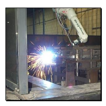
Welding, in general, is a process that lends itself well to automation for suitable part geometries. Robotic welding is fast, repeatable, and best suited to long-run production.
